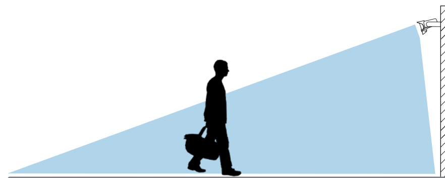
Senstar MultiSensor is installed tilting downwards at an approximate 20° angle, 2.4 to 3.7 m (8 to 12 ft) above the ground.
