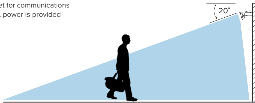
Senstar MultiSensor is installed tilting downwards at a 20° angle, 2.4 to 3.7 m (8 to 12 ft) above the ground.
