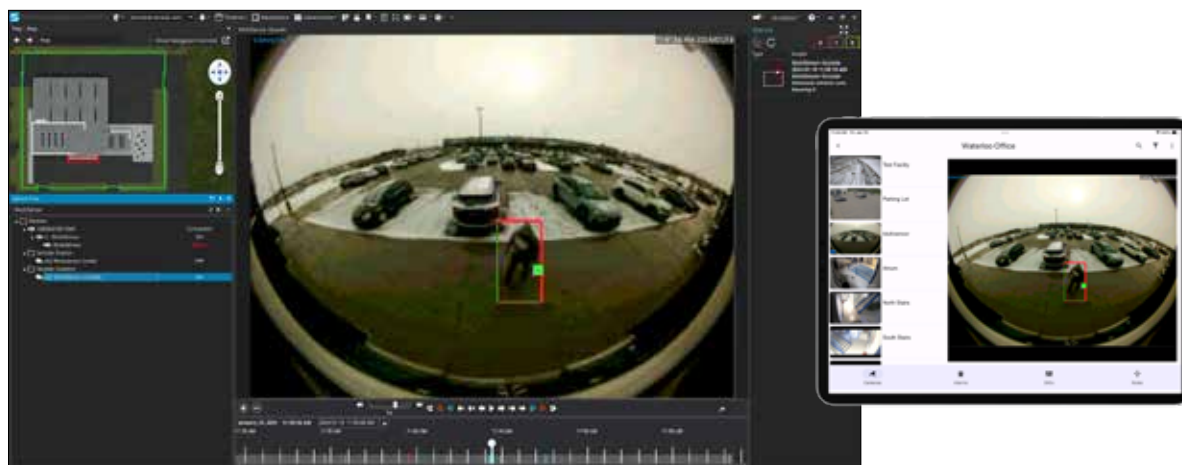
Senstar MultiSensor, connected to the Senstar Symphony Common Operating Platform, empowers users with real-time, critical information, including intrusion data and image capture.
