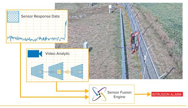
Sensor Fusion Engine detecting a daytime fence climb. In this example, the engine is using video from a any ONVIFcompatible surveillance camera (include low-light and thermal). Data from an deep-learning trained video analytic is synthesized with live and historical fence response data from a FlexZone processor to intelligently characterize the risk (valid intrusion attempt). Intruder
