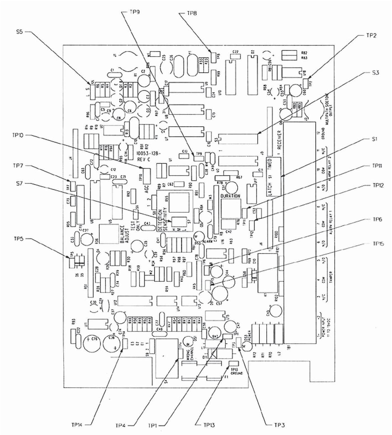
Figure 17. Receiver Circuit Board Component Location
