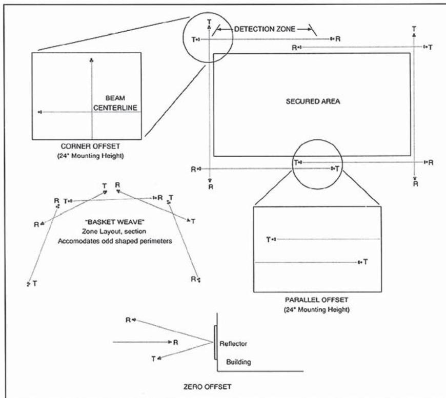
Figure 8: Offset Arrangements: Typical High Security Installation
