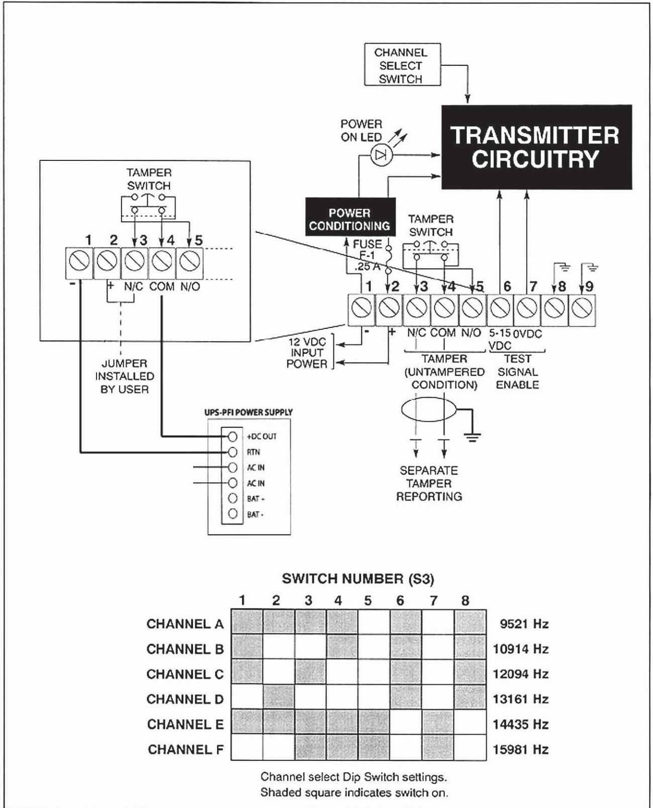
Figure 11: Transmitter Wiring
