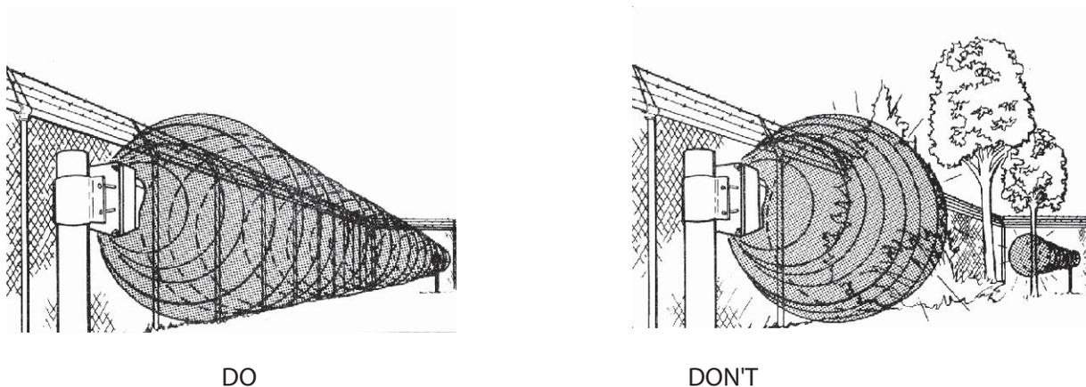
**Figure 3. Required Clearance Area**
