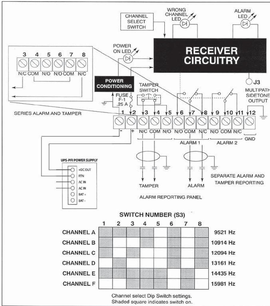
**Figure 12. Receiver Wiring**
