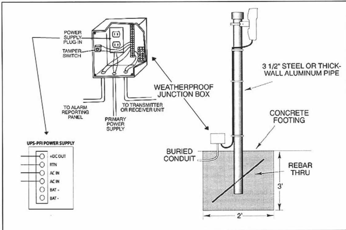
**Figure 9. Post Installation and Mounting Units**
