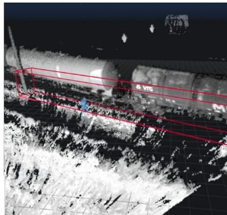
With 3D LiDAR, security systems can monitor volumetric zones around trains, tracking activity in all three dimensions.
