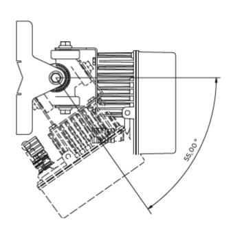
Drawing depicts most restrictive configuration. Max. pan angle in opposite direction: 75°. Dimensions in mm Values in brackets are calculated and may contain round-off errors
