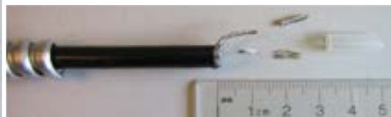
Figure 54: Armored cable preparation for splicing
