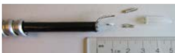
Figure 58: Armored cable preparation for terminations
