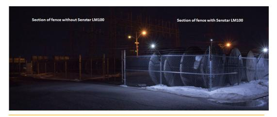
This image shows the difference between a fence with the Senstar LM100 and one without
