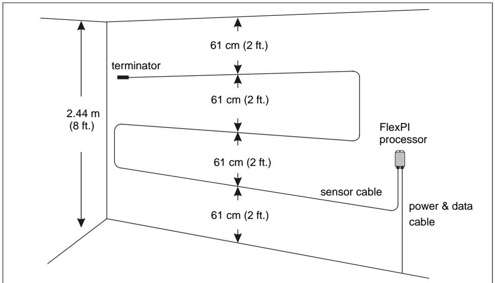
Figure 3: High-security application (triple pass on 8 ft. wall)
