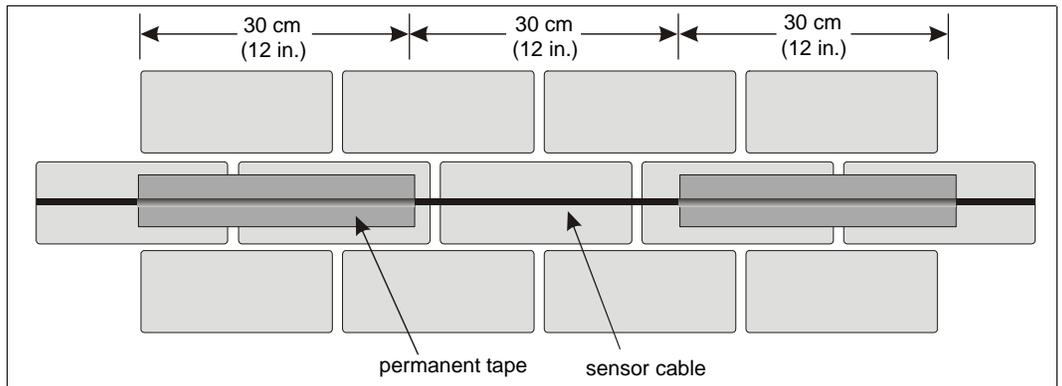
Figure 14: Installing sensor cable with permanent tape
