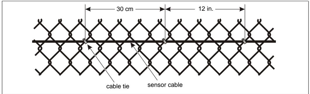
Figure 11: Mounting sensor cable on security cages/fences
