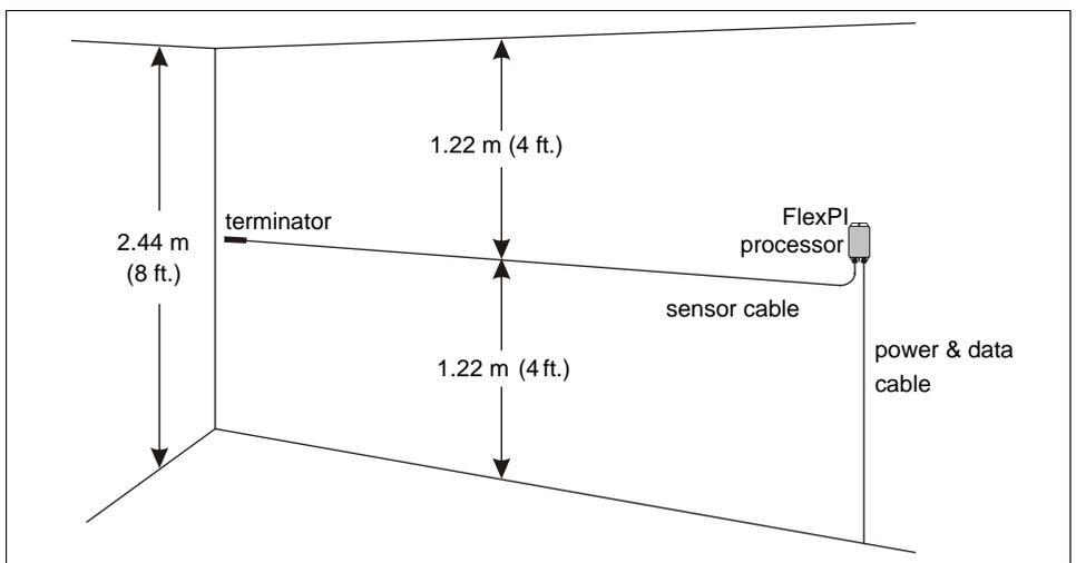
Figure 5: Low-security application (single pass on 8 ft. wall)
