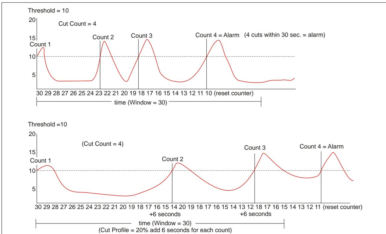
Figure 29: Understanding the Cut Alarm
