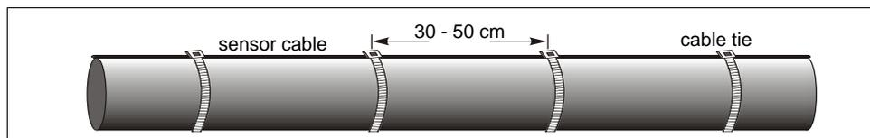
Figure 8: Protecting pipelines
