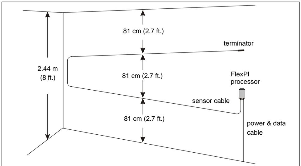
Figure 4: Medium-security application (double pass on 8 ft. wall)
