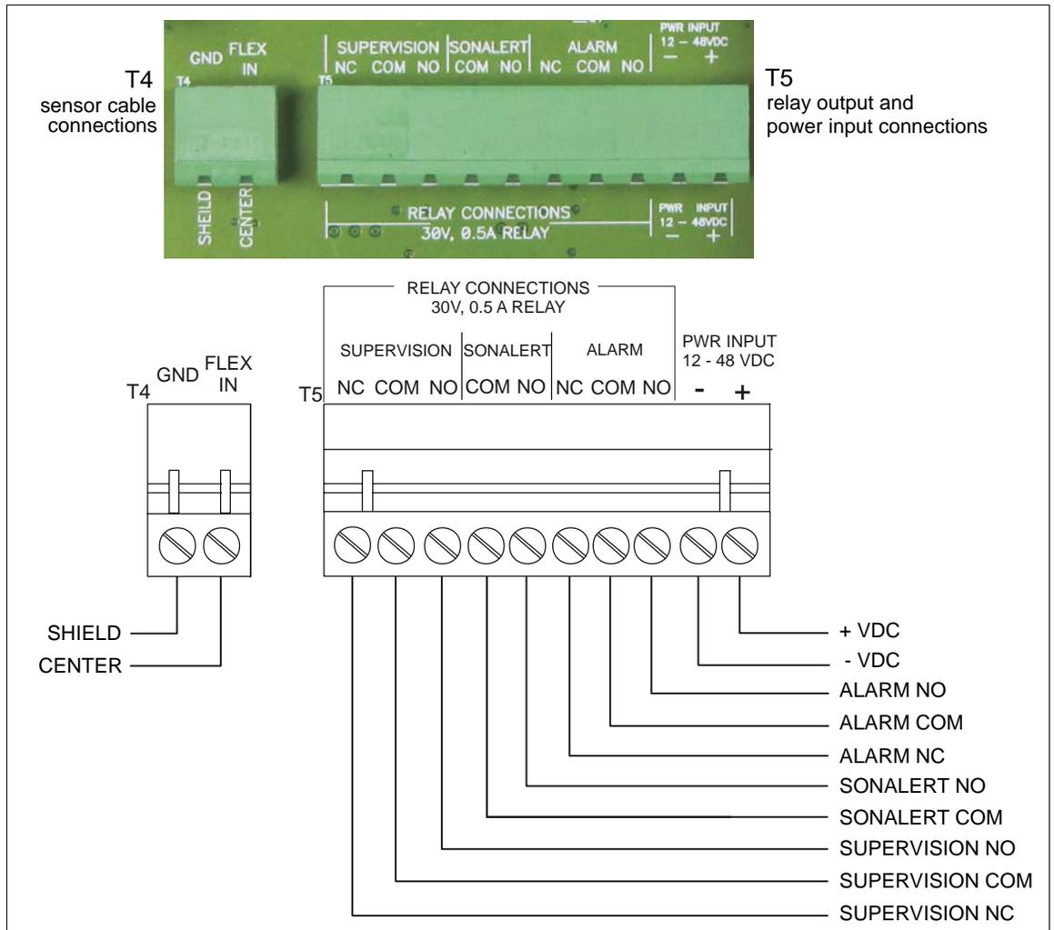
Figure 24: FlexPI wiring diagram
