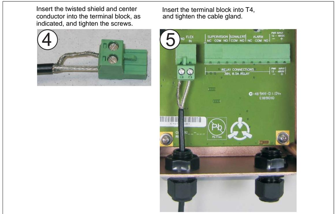
Figure 22: Connecting the sensor cable/lead-in cable
