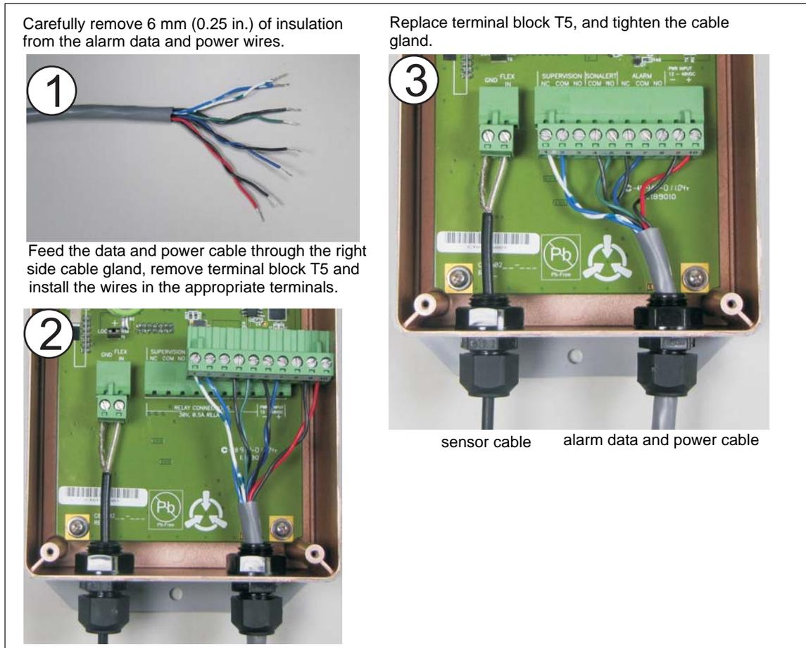
Figure 23: Connecting the data and power cables
