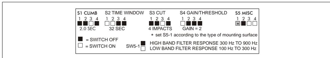
Figure 27: Recommended switch settings
