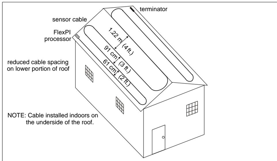
Figure 7: Roof protection
