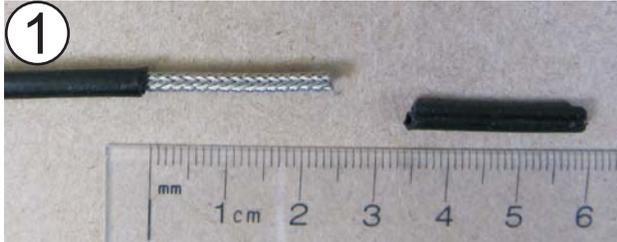
Tightly twist the strands into a single conductor, and then carefully remove 6 mm (0.25 in.) of insulation from the center conductor. DO NOT nick the center conductor.
