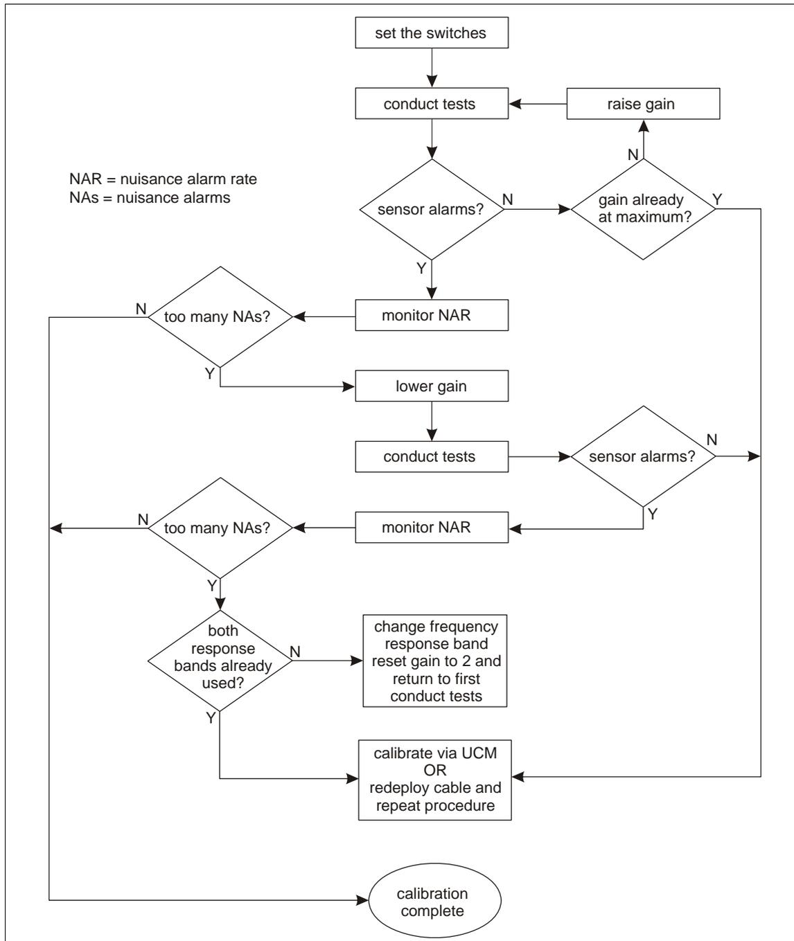
Figure 28: Gain/Threshold setting flow chart
