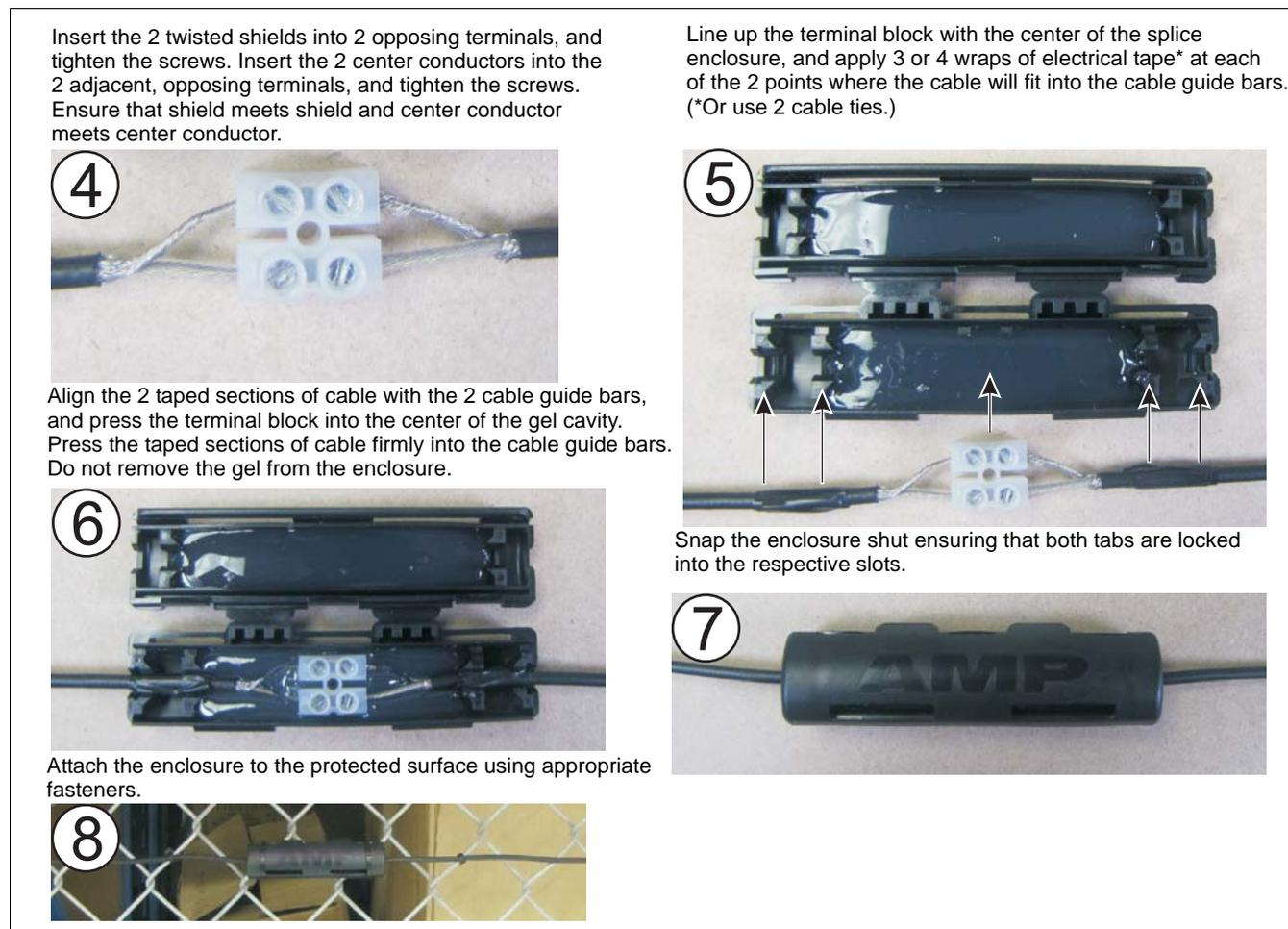
Figure 18: Splice-connecting sensor cable
