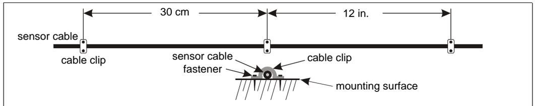
Figure 13: Mounting sensor cable on walls/flat surfaces
