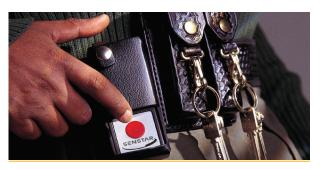
The PPDs are easy-to-use devices that instantly send a call for help at the press of a button. The belt-holster includes pull-pin activation and man-down options.
