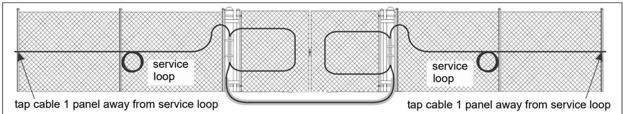
Figure 104 Tap test location - gate (part of zone)
