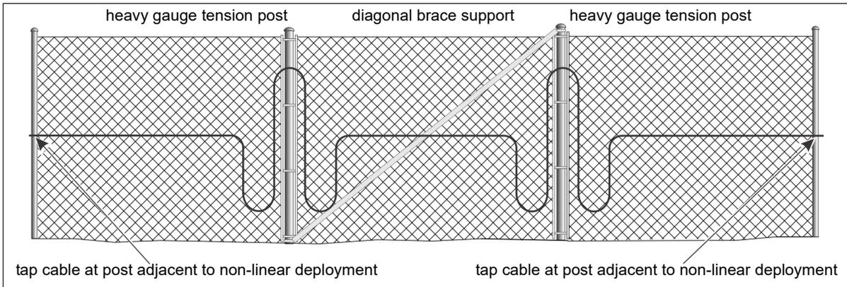
Figure 106 Tap test location - non-linear cable deployment
