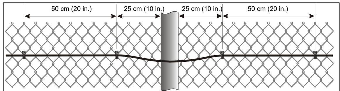
Figure 50 Cable tie spacing at fence posts
