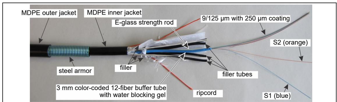
Figure 8 FiberPatrol armored sensor cable (FPSP0624)
