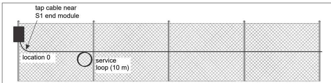
Figure 96 Tap test location - Set Start (Split configuration)
