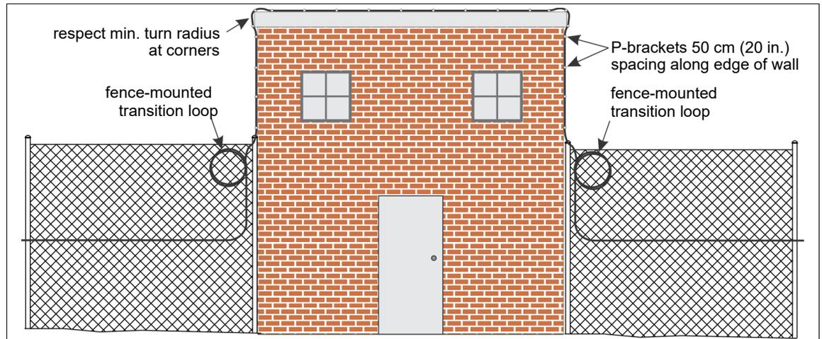
Figure 28 Protecting a masonry structure along the perimeter
