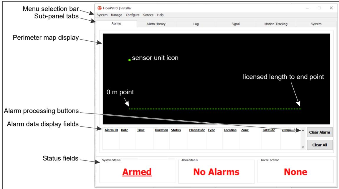
Figure 85 FiberPatrol default Alarm screen (installer access level)
