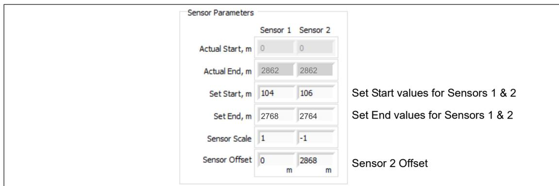
Figure 94 Calibrated Sensor Parameters (from examples above)
