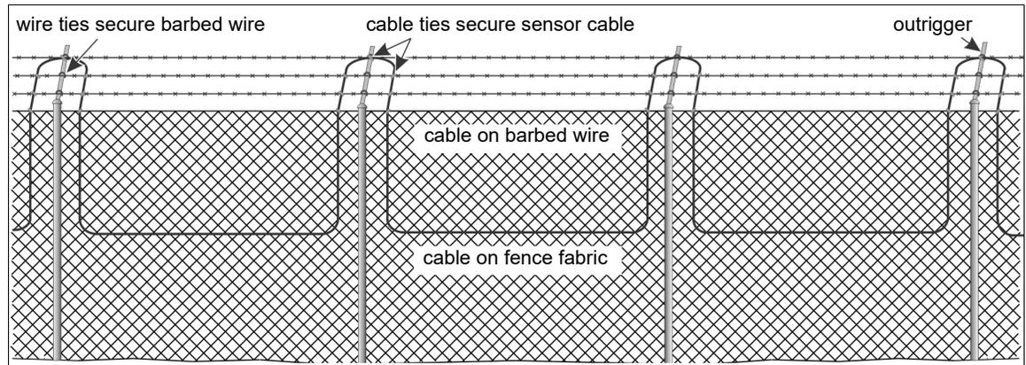
Figure 21 Sensor cable installation on barbed wire fence
