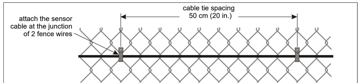
Figure 49 Cable tie spacing on fence fabric
