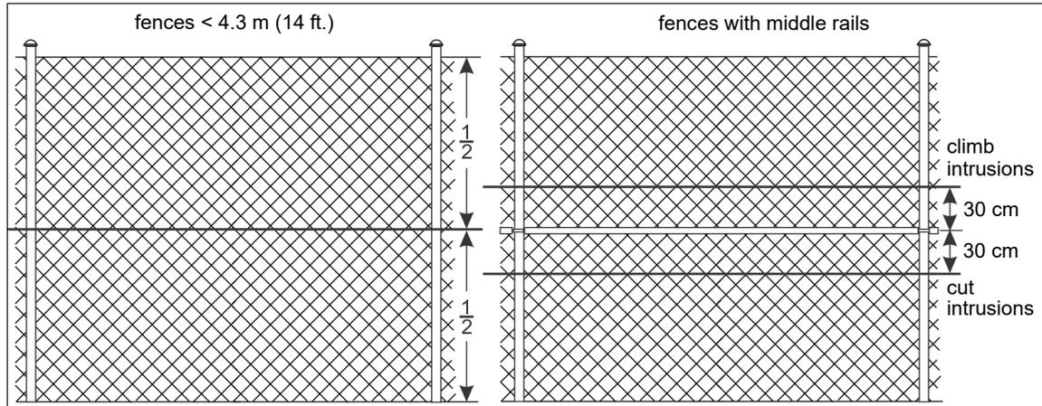
Figure 20 Recommended fence height/cable pass configurations
