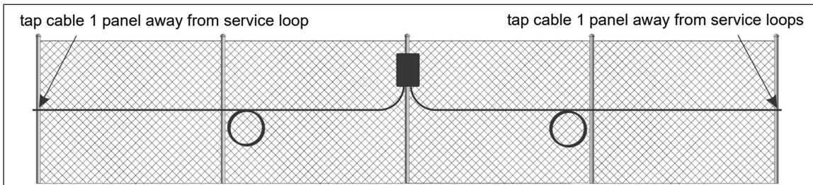
Figure 100 Tap test location - outdoor splices
