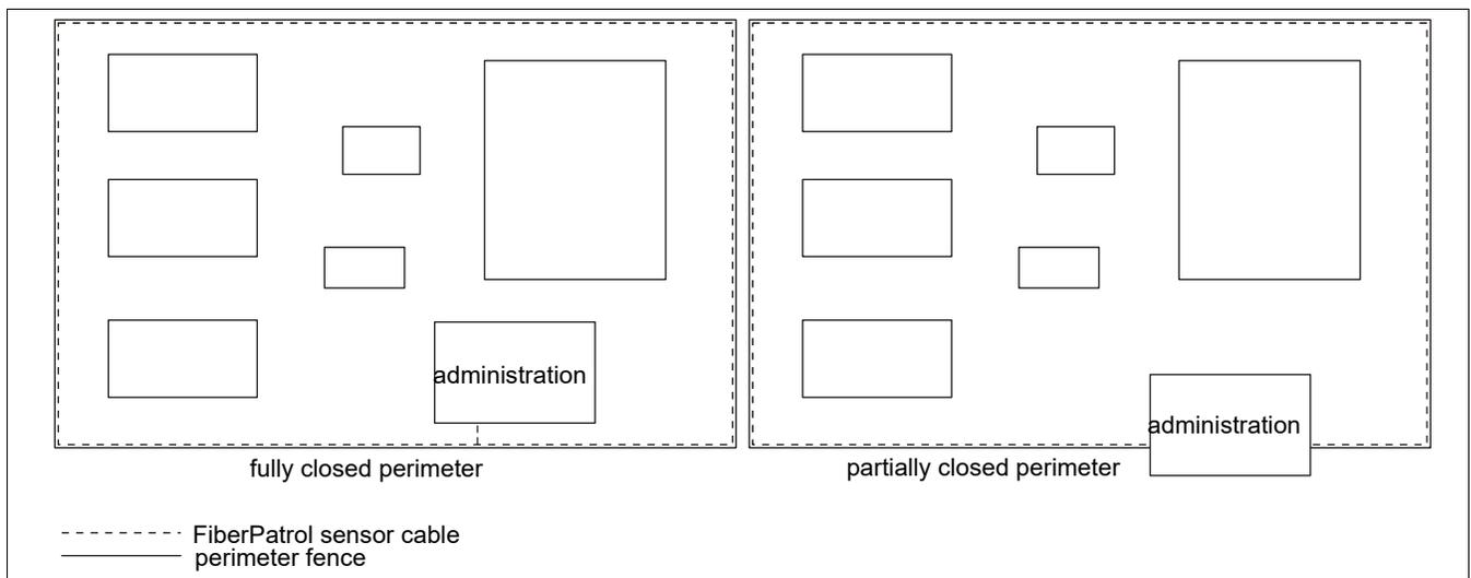
Figure 11 FiberPatrol example fully closed & partially closed configurations
