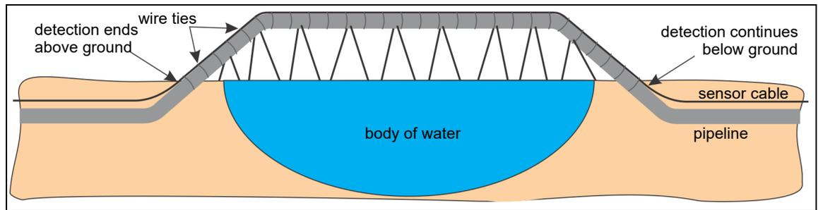
Figure 47 Sensor cable bypass (body of water)
