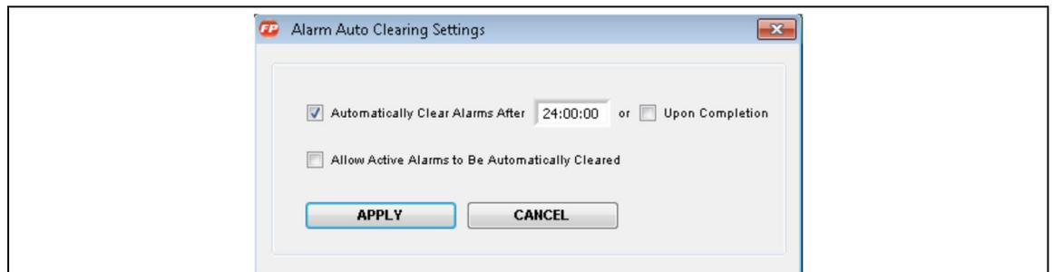
Figure 153: FiberPatrol Alarm Auto Clearing Settings
