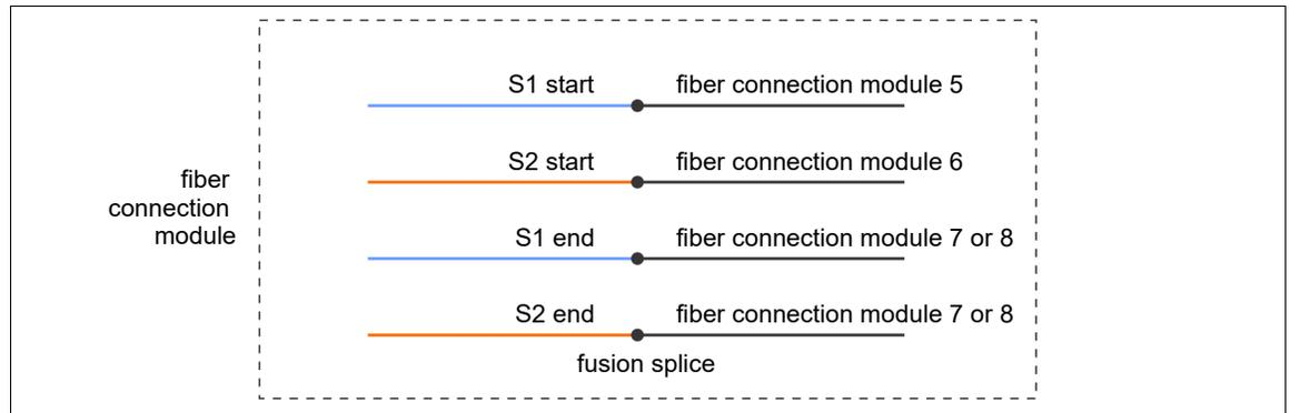
Figure 72 Sensor cable fiber splicing connections
