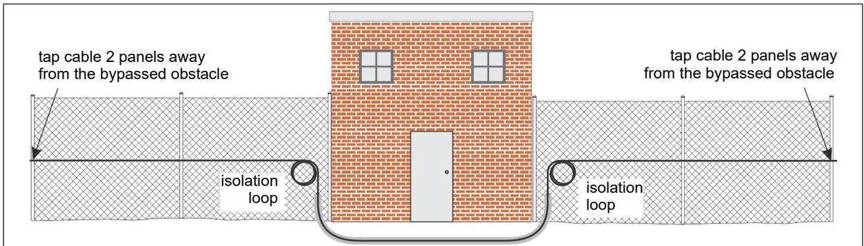
Figure 105 Tap test location - bypassed obstacles
