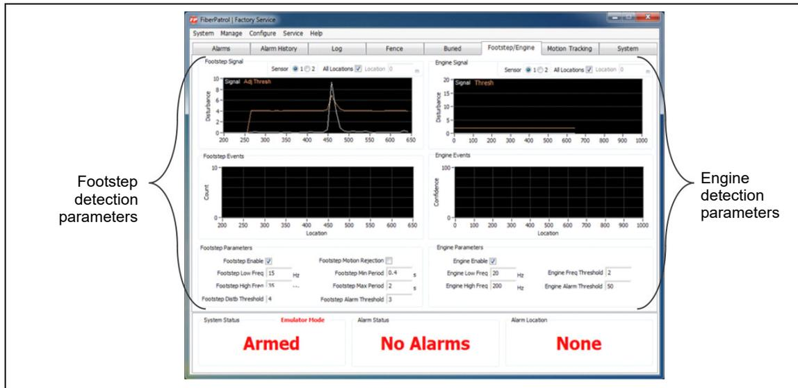
Figure 147: Footstep/Engine Sub-panel
