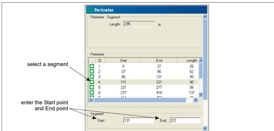
Figure 119 Defining the positions of the perimeter segments
