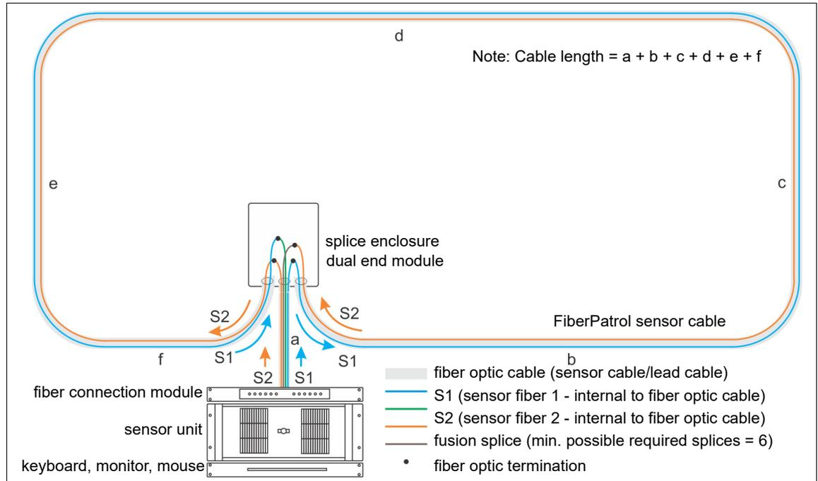
Figure 14 FiberPatrol fully closed redundant loop configuration
