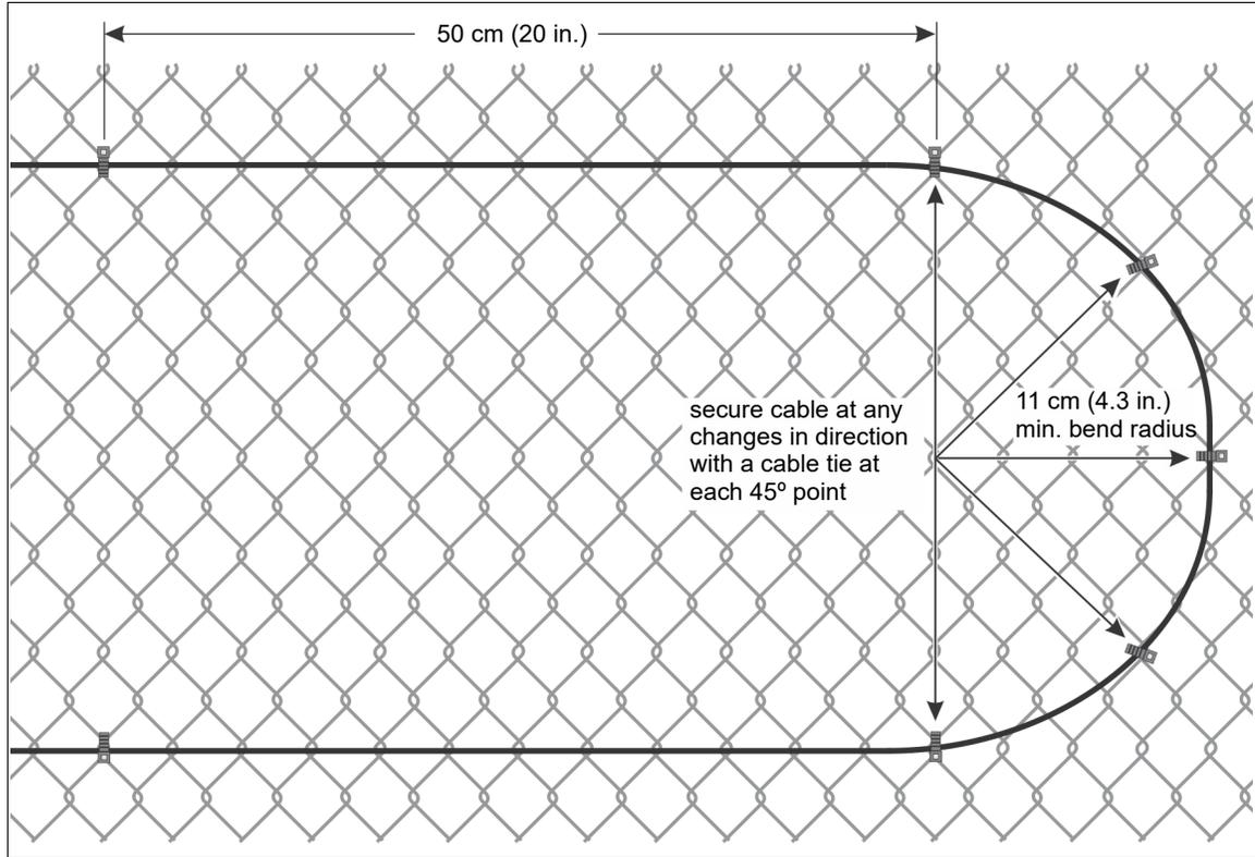
Figure 51 Cable tie spacing around corners
