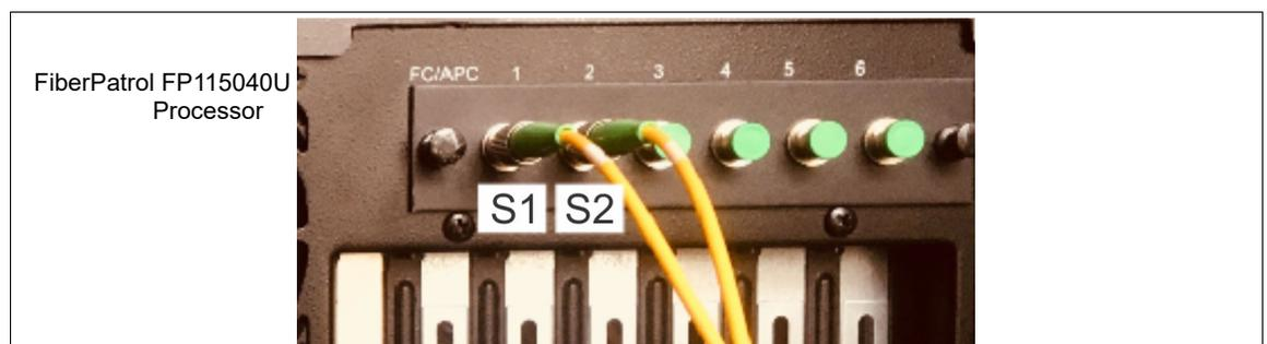
Figure 74 FP115040U fiber connections
