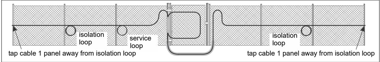
Figure 102 Tap test location - gate (independent zone)
