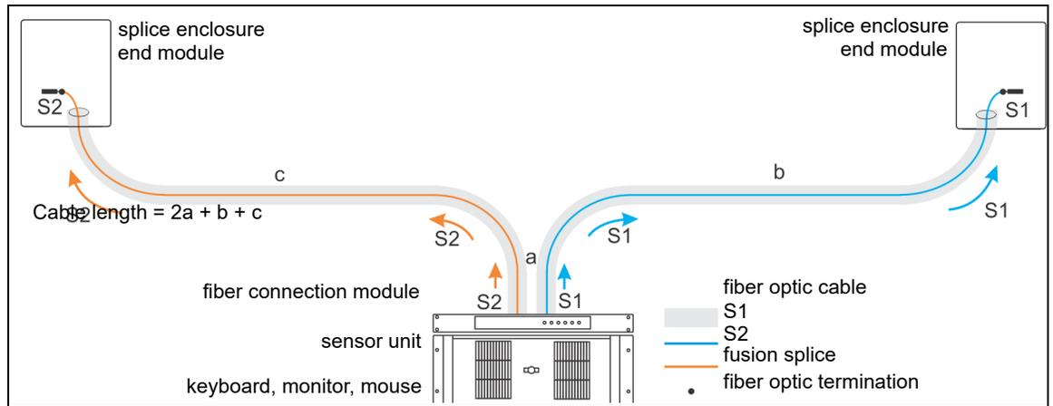
Figure 17 FiberPatrol split configuration (2 lead cables)
