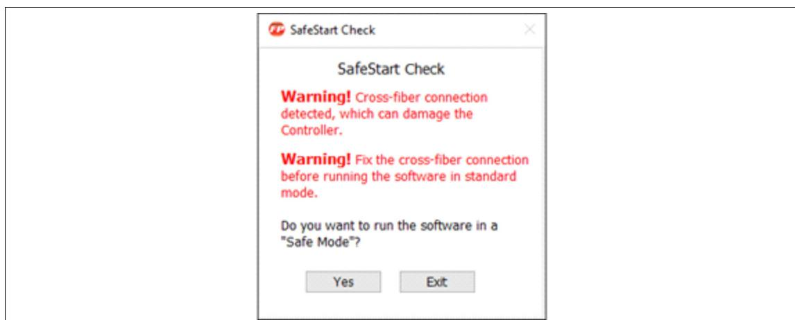
Figure 83 Cross-fiber detected
