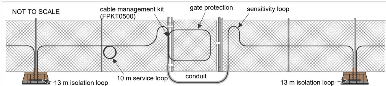
Figure 27 Independent gate zone (with buried isolation loops)
