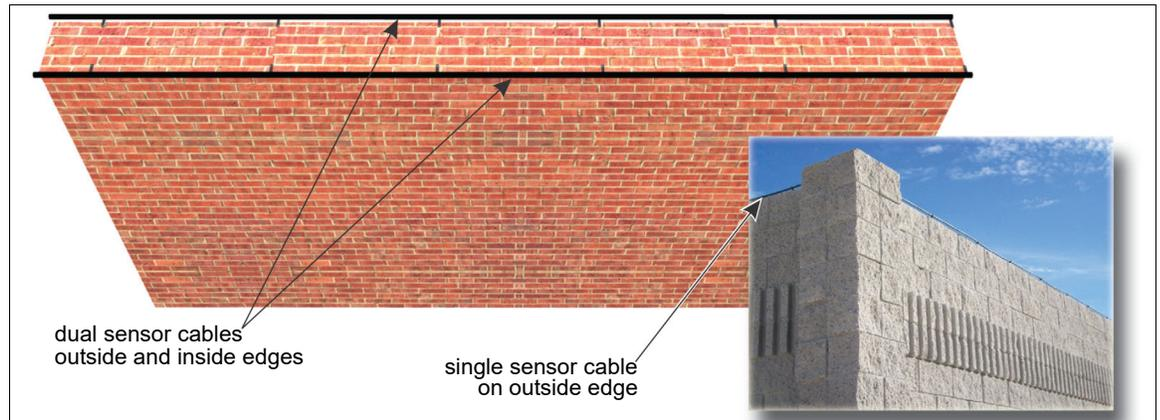
Figure 29 Protecting a masonry structure along the perimeter
