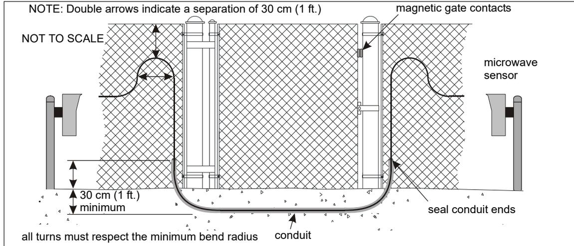
Figure 23 Gate bypass
