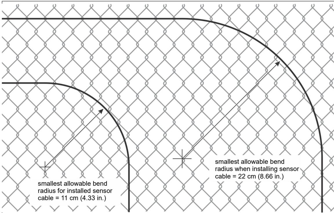
Figure 52 Static and dynamic bend radius limits
