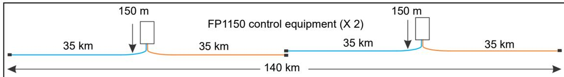
Figure 48 Example length calculation drawing
