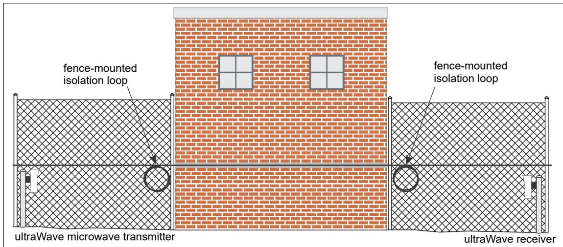
Figure 35 Perimeter structure bypass (through structure)
