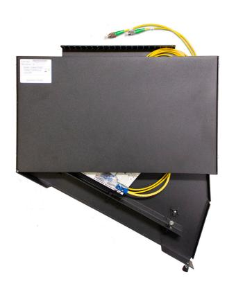
The 1U rack-mount enclosure is used to house the dual end modules for the FP1150 and enables the splicing of field cable to patch cords (for connection to the FP1150 processor). The module is designed for installation in a 19-inch rack. The slide-out tray provides easy access to the optical module to facilitate field splicing.
