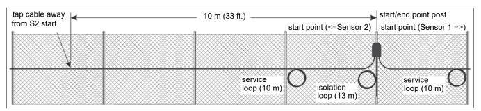
Figure 13 Tap test location - Set Start Sensor 2 (fully closed loop example)
