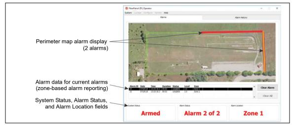
Figure 58 FP1400 series Operator Alarms panel (2 alarms)
