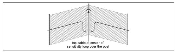
Figure 22 Tap test location - at corners or heavy gauge posts
