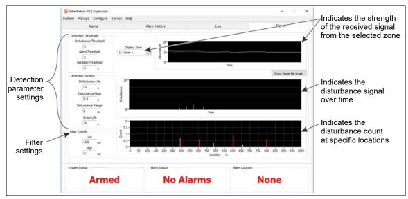
Figure 66: Signal sub-panel
