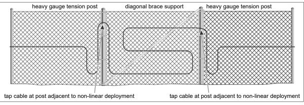
Figure 27 Tap test location - non-linear cable deployment
