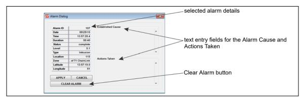
Figure 61 FiberPatrol Alarm Dialog
