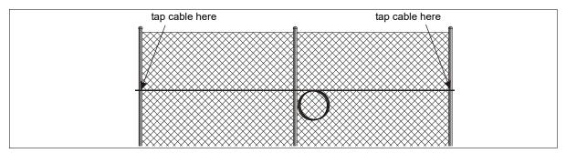
Figure 28 Tap test location - service loops
