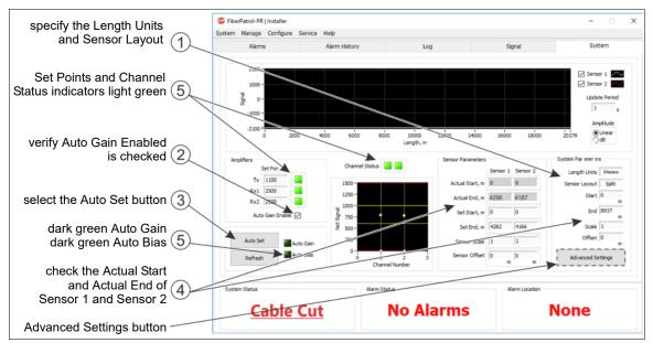
Figure 7 FiberPatrol System configuration (installer access level)
