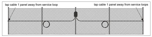
Figure 21 Tap test location - outdoor splices
