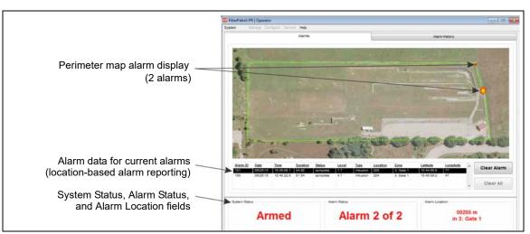
Figure 57 FP1100X series Operator Alarms panel (2 alarms)
