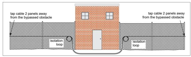
Figure 26 Tap test location - bypassed obstacles
