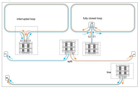
Figure 6 FiberPatrol sensor cable configurations
