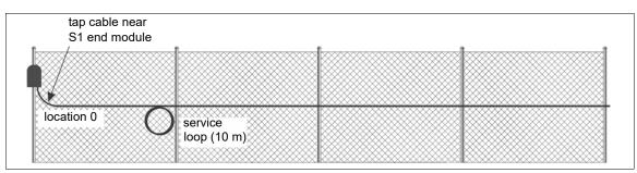
Figure 16 Tap test location - Set Start (Split configuration)
