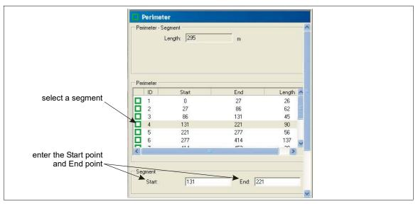
Figure 39 Defining the positions of the perimeter segments
