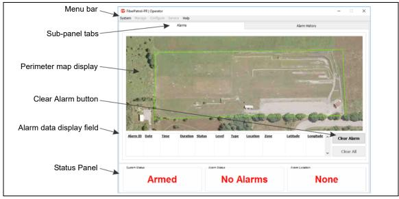
Figure 56 Operator Control panel (no alarms)
