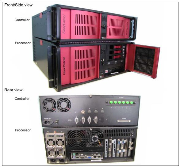
Figure 1 FiberPatrol processor & controller
