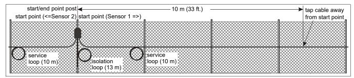
Figure 11 Tap test location - Set Start Sensor 1 (fully closed loop example)
