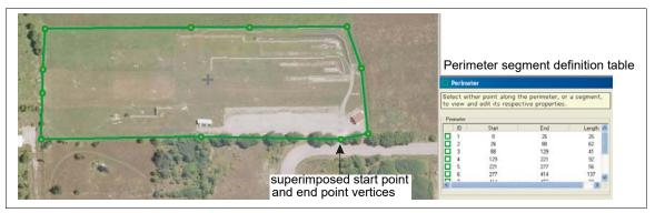
Figure 38 Drawing the perimeter
