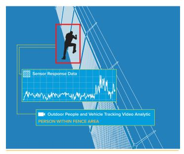
The Sensor Fusion Engine intelligently synthesizes low-level data from fence sensors and video analytics to provide the highest possible level of protection while generating fewer nuisance alarms when compared to using just a fence sensor, an outdoor video analytic, or even a boolean logic integration of the two.
