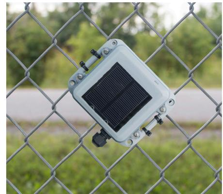
The Senstar Wireless Gate Sensor eliminates the need to run sensor or power cables onto a moving gate panel. It uses 128-bit AES encrypted communications and includes supervision mechanisms that generate alarms if the device is physically moved or damaged, or if the RF communications link is in some way compromised. It also guards against replay and cloning attacks.
