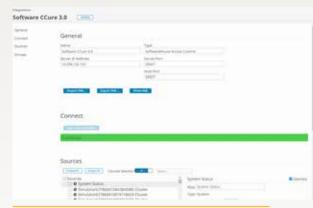
Configuration of the Software House CCure 9000 is performed within Senstar Symphony's web-based setup, making configuration quick and easy.
