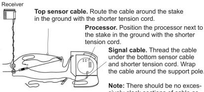
Signal cable. Thread the cable
