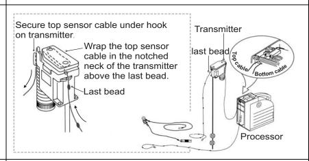
7 Attach the **bottom sensor cable** to the cleat on the short tension cord.
