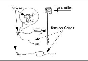
Attach the **shorter tension cord** with a cleat to one of the stakes in the ground. Do not attach the cleat end of the shorter tension cord to the stake or anchor. You attach the cleat end of the shorter tension cord to the bottom sensor cable.
