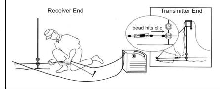
Remove the receiver from the storage area on the processor chassis. Attach the receiver to the last support pole on the perimeter.
