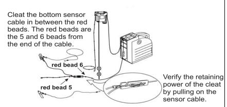
Set the height of the **bottom sensor cable support** to 15 cm (6 in.) above the ground.
