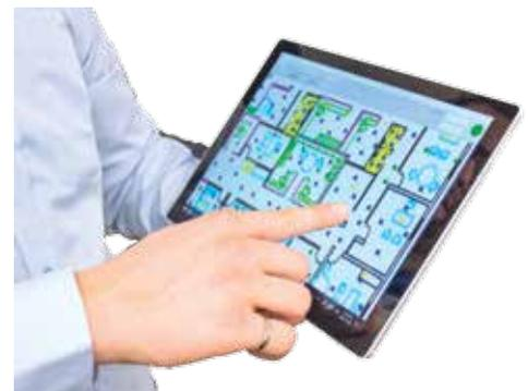
Calibration and system verification is quickly performed with Senstar’s tablet-based software. The streamlined process minimizes disruptions to daily operations and ensures that there are no coverage dead zones.
