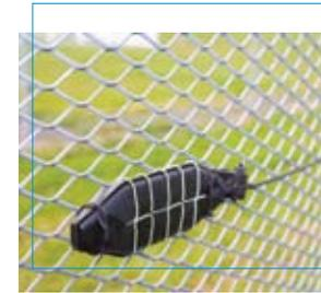
**IntelliFIBER™** is a fence-mounted sensor that uses the signals generated by the minute flexing of a proprietary fiber optic sensor cable to detect an intruder cutting, climbing, or lifting the fence fabric. It is particularly useful where there is a risk of EMI, RFI or lightning.
